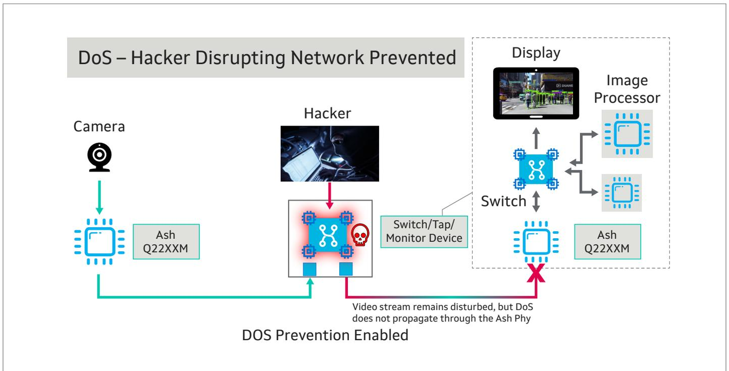
Figure 6f: DoS data from hacker is dropped by Ash PHY connected to Image processing sub-system due to key mismatch.
